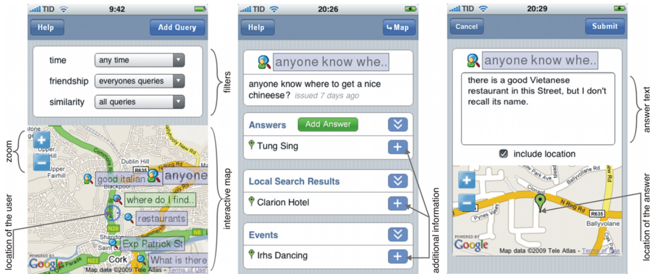
Figure 1. Screenshots of the SocialSearchBrowser (SSB) Application: (left) The map screen is the main screen of the SSB application. Queries are overlaid on a Google maps visualization (own queries are show with a green semi-transparent background) and three drop down menus that allow the user to filter the displayed queries; (center) The query detail screen shows three categories of answers: (1) answers by other users, (2) results from Google local search and (3) results from Eventful API; (right) When a query is answered, the user can optionally add a location.
